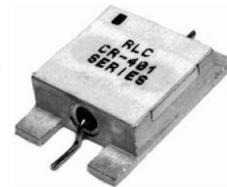
RLC Electronics' miniature surface mount detectors utilize a zero-bias Schottky design. The microwave power is coupled directly to the extremely small components reducing package parasitics and transition mismatches. This design results in a low VSWR and a flat, smooth output over a wide bandwidth. Standard unit has frequency range of .01 to 4 GHz, with option of negative or positive output. A higher frequency option is available up to 12.4 GHz.
