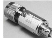
RLC Electronics' Zero Bias Detectors are designed for use in coaxial systems in the measurement of relative microwave power up to 100 mW over the frequency range of 10 MHz to 18.0 GHz. The design assures flat frequency response combined with high sensitivity. Options available include negative output polarity, positive output polarity, matched pairs, and Square Law response.
