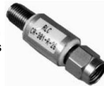
RLC Electronics' miniature ultra-flat detectors utilize a zero-bias Schottky design. The microwave power is coupled directly to the extremely small components reducing package parasitics and transition mismatches. This design results in a very low VSWR and a flat, smooth output over a wide bandwidth. Options available include negative or positive output, a choice of three output connectors and operation to 26.5, 40 GHz or 43.5-45.5 GHz.
