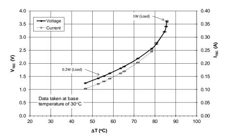
Note that  $\Delta T$  is difference between the temperature of the detector and that of the base, the TO-8 header and stud. This is typically warmer than the ambient environment. Good performance requires the base to be kept as cold as feasible. Note that the power drawn by the cooler decreases rapidly with  $\Delta T$ . If maximum cooling ( $\Delta T = 85$  °C) occurs at 1 W, at 0.5 W  $\Delta T$  is about 78 °C, and at 0.2 W,  $\Delta T$  is 55 °C.
