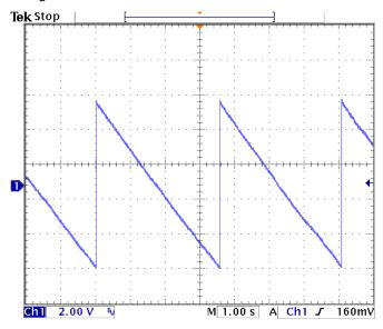
**Preamplifier output.** This trace also shows the preamp output but on a different voltage and time scale to illustrate the reset. The small steps from each signal integrate towards the negative rail, where a reset signal is generated. This results in a sawtooth of several volt amplitude. The period depends on the total current through the detector (signal current plus leakage current).
