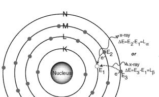
3a) When a vacancy is created in the L shell by either the primary excitation x-ray or by the previous event, an electron from the M or N shell "jumps in" to occupy the vacancy. In this process, it emits a characteristic x-ray unique to this element and in turn, produces a vacancy in the M or N shell.
