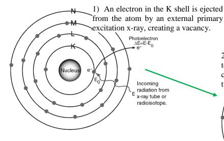
2) An electron from the L or M shell "jumps in" to fill the vacancy. In the process, it emits a characteristic x-ray unique to this element and in turn, produces a vacancy in the L or M shell.
