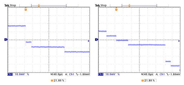
**Preamplifier outputs.** These traces illustrate typical output pulses with a SiPIN detector, measured using 5.89 and 22.1 keV X-rays. Each X-ray interaction results in a negative going step of ~1 mV/keV.
