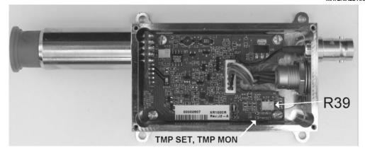
The figure above shows how to adjust the controller on the XR-100CR. Remove the top cover and adjust the R39 pot to achieve the desired TMP SET value. This is the set point temperature. It reads in mV with the calibration curve shown in the next section. TMP MON shows the measured temperature in mV with the same calibration curve.
