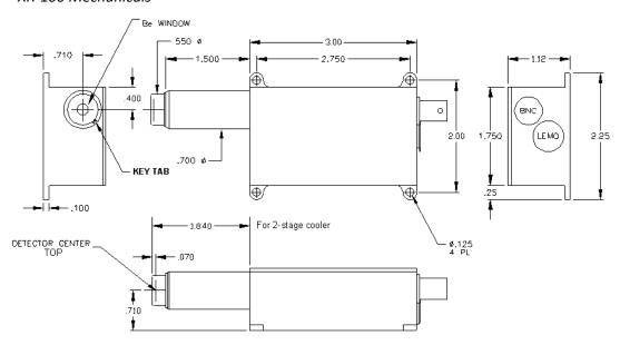
Mechanical design of standard XR-100 (1.5" extender). Visit <u>www.amptek.com</u> or contact Amptek for dimensions of the other configurations (5" extender, 9" extender, etc.).
